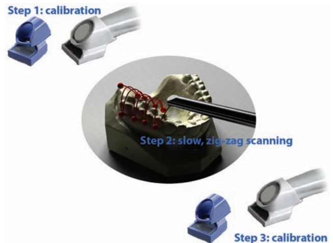
Figure 4. The hi-res scanning protocol for the Lava COS scans. The scanning protocol for the scans for the Lava COS is the normal scanning protocol, except that the scan-path is a slow zigzag scan and that at the end of the scan a second calibration is performed.
